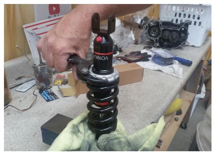
Turn the preload ring a half revolution, then snug up the lock ring. Temporarily re-install the shock and seat, and test how the adjustment feels. Repeat this process as necessary to achieve the correct feel for you, but do NOT exceed more than 10mm of exposed thread beneath the lock ring. This is the best way to set your preload: once you have it set to your liking, it's unlikely you will adjust it further in the future.
