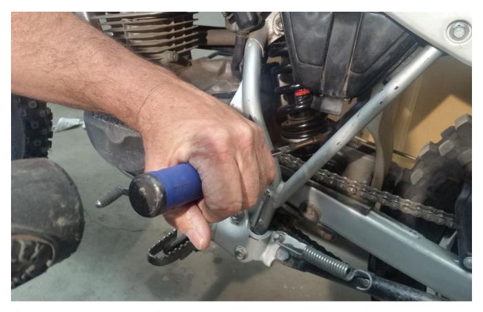
It's possible to adjust the preload after the shock is installed, but access is limited, and you need to use the correct tool. We recommend the brass-tipped preload punch from Motion Pro (model 08-0483): the brass tip is softer than the aluminum preload/lock rings, which prevents damage. We strongly advise against using a standard punch or screwdriver to do this adjustment. Before doing any adjustment, be sure to loosen the lock ring. After adjusting, don't forget to snug the lock ring back up.
